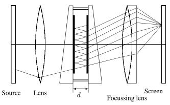
The width of the peaks at half height is given by  $\gamma = 4/\sqrt{F}$ . The finesse  $\mathcal{F}$  is defined as  $\mathcal{F} = \frac{1}{2}\pi\sqrt{F}$ . The maximum resolution is then given by  $\Delta f_{\min} = c/2nd\mathcal{F}$ .
