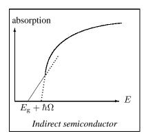
So indirect semiconductors, like Si and Ge, cannot emit any light and are therefore not usable to fabricate lasers. When light is absorbed holds:  $\vec{k}_{\rm h} = -\vec{k}_{\rm e}, \, E_{\rm h}(\vec{k}_{\rm h}) = -E_{\rm e}(\vec{k}_{\rm e}), \, \vec{v}_{\rm h} = \vec{v}_{\rm e}$  and  $m_{\rm h} = -m_{\rm e}^*$  if the conduction band and the valence band have the same structure.
